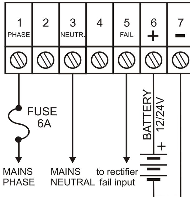
**PHASE INPUT:** This is the power supply input for the battery charger. Please see technical specifications for ratings. A fast type fuse should be used in series with this input.
