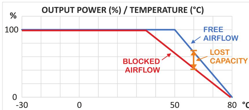
**Preventing airflow will reduce the charger rating in high temperature.**
