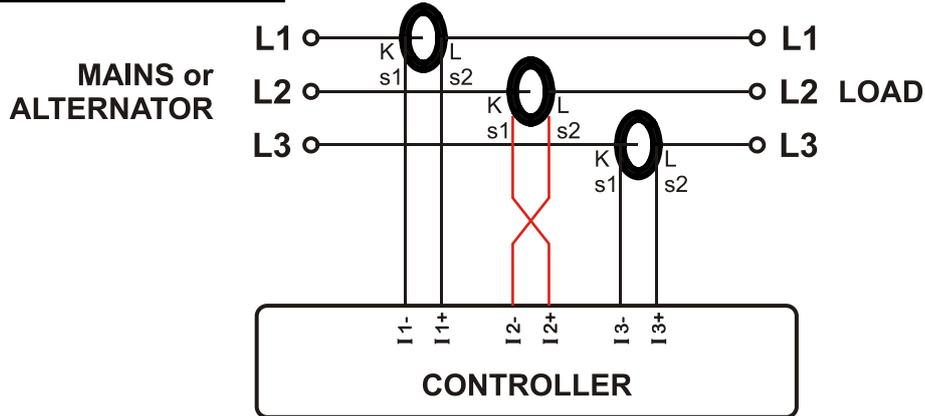
The generator is still loaded with 100 kW On each phase. The load Power Factor (PF) is 1. PF in phase L2 will show -1,00 due to reverse CT polarity. The result is that total generator power displayed by the controller is 100 kW. Measured values are as follows:
