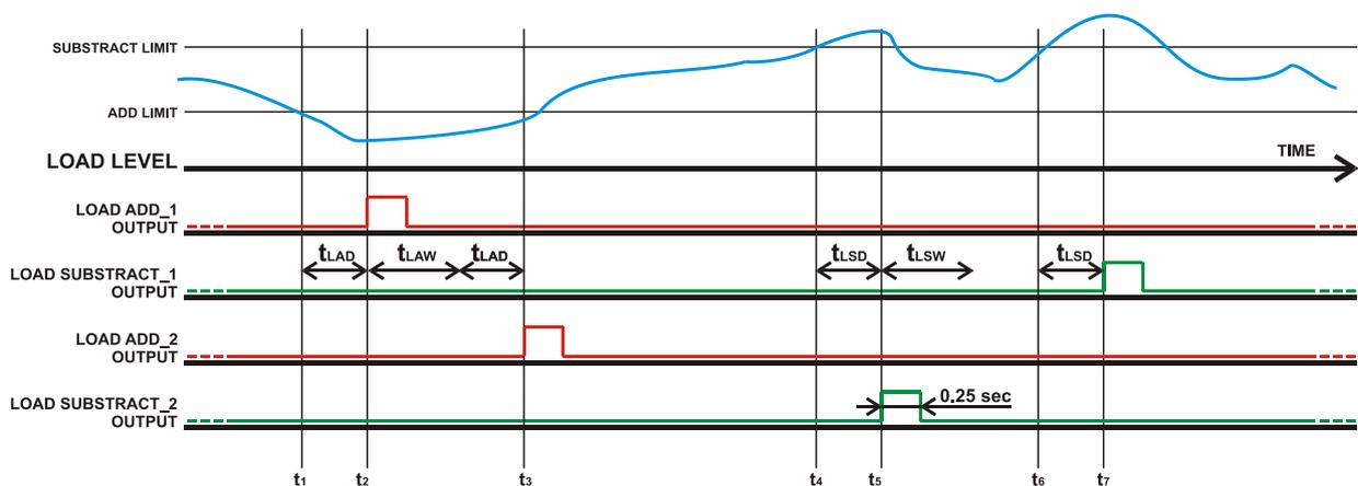
**t1:** the load goes below the Multi Load Add Power Level.
