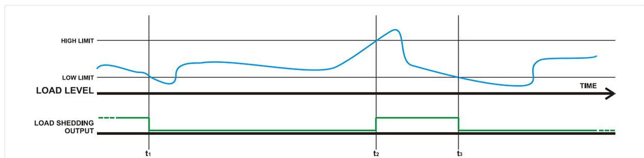
**t<sub>1</sub>:** the load goes below the Load Shedding Low Limit, thus the Load Shedding output becomes inactive.
