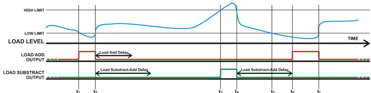
**t<sub>1</sub>:** the load goes below the Load Shedding Low Limit, thus the Load Add output becomes active.
