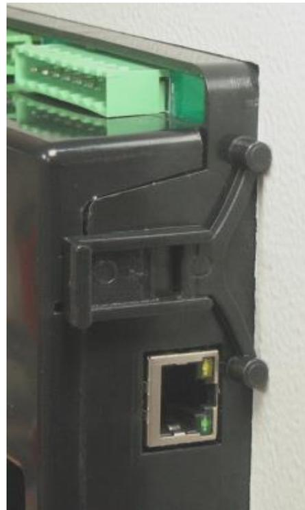
Installation of self retaining type bracket
