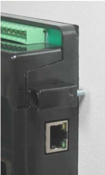
Installation of screw type bracket
