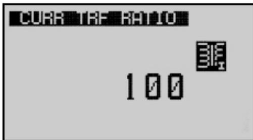
For the correct current measurement, the current transformer ratio has to be set properly. The secondary of the current transformer is always supposed to be 5 Amps. Only the primary value is set. Select “**CRNT TRF RATIO**” on “**CONFIGURATION MENU**”.
