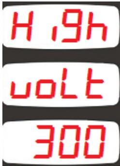
This parameter adjusts the upper limit of the high voltage alarm.
