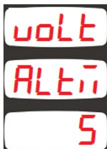
This parameter determines the delay between a high or low voltage alarm condition occurs and the alarm given.
