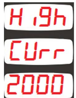
This parameter adjusts the overcurrent limit.
