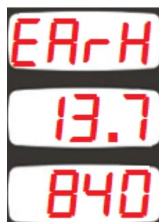
In earth leakage input calibration mode, the first display will show "EARH". The second screen will display the measured instantaneous voltage from the input. The third display will display the calibration coefficient (high 4 digits only)
