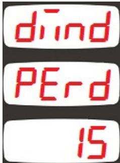
This parameter determines the demand period for voltage, current and power measurements. The average value is calculated during the demand period and at the end of the period new demand values overwrite older values.
