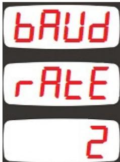
This parameter determines the data rate (baud rate) used in the Modbus communication. Every unit in the same Modbus loop must use the same data rate.
