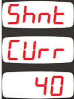
This parameter adjusts the rated value of the current shunt in amperes.
